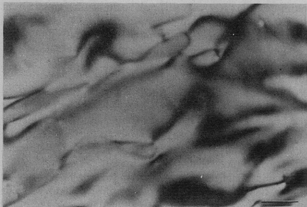
Figure 2. Thin layer of anisotropic phase of I viewed in polarized light. The appearance is of a typically nematic structure. The bar is 600 \mu\text{m} .
